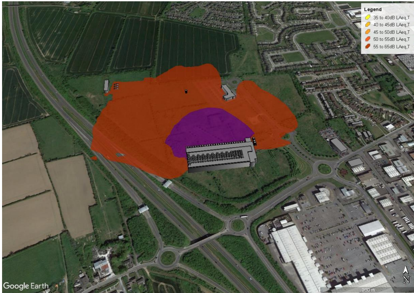
Figure 10.6 Scenario B Proposed Development and Permitted Data Storage Facility– Emergency Noise Contour (Extent of 55dB(A))
