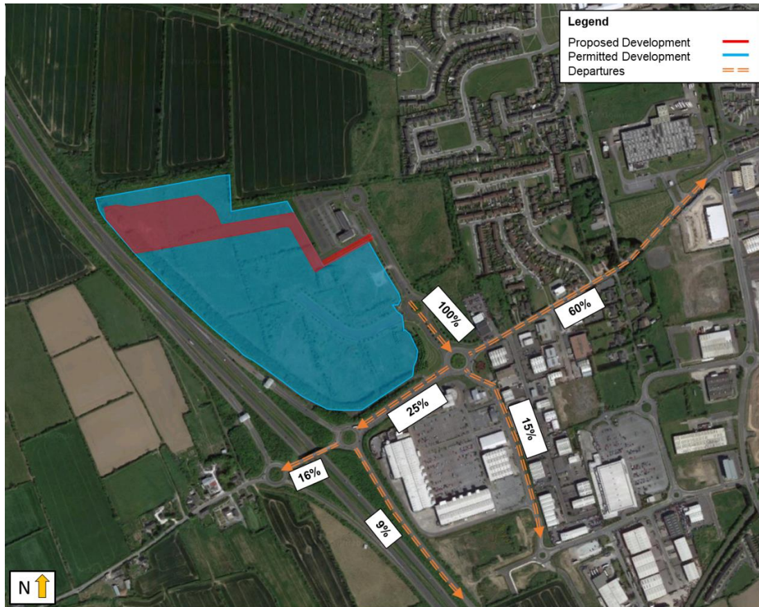
Figure 13.7: Proposed Development Departures Turning Proportions--Construction phase
