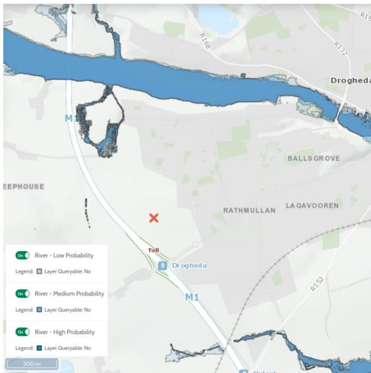
Figure 5.2 CFRAM Fluvial mid-range future scenario flood map. Site located at red X (OPW, 2019)
